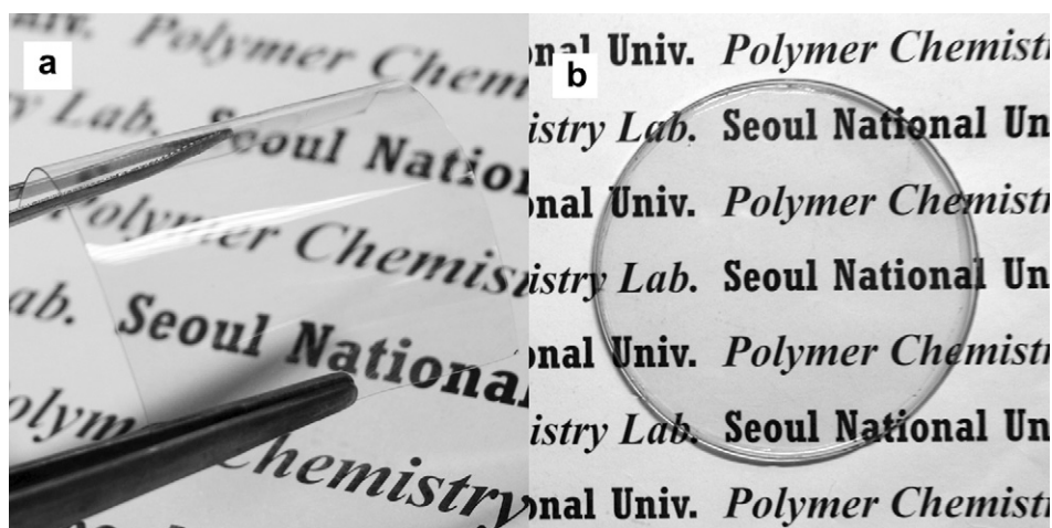
Fig. 3. Photo images of free standing polymer films, (a) PES20 and (b) PES25, obtained by casting from THF solution.
